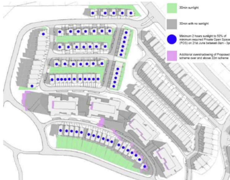
Figure 26 Compliant v non-compliant solar access, 12pm (Source: Mirvac Design)
