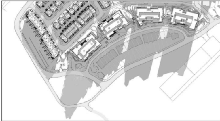
Figure 24 Shadow diagram, 3pm (Source: Mirvac Design)
