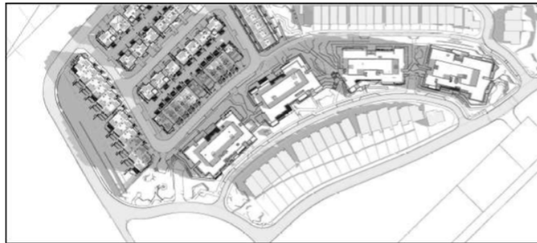
Figure 22 Shadow diagram, 9am (Source: Mirvac Design)
