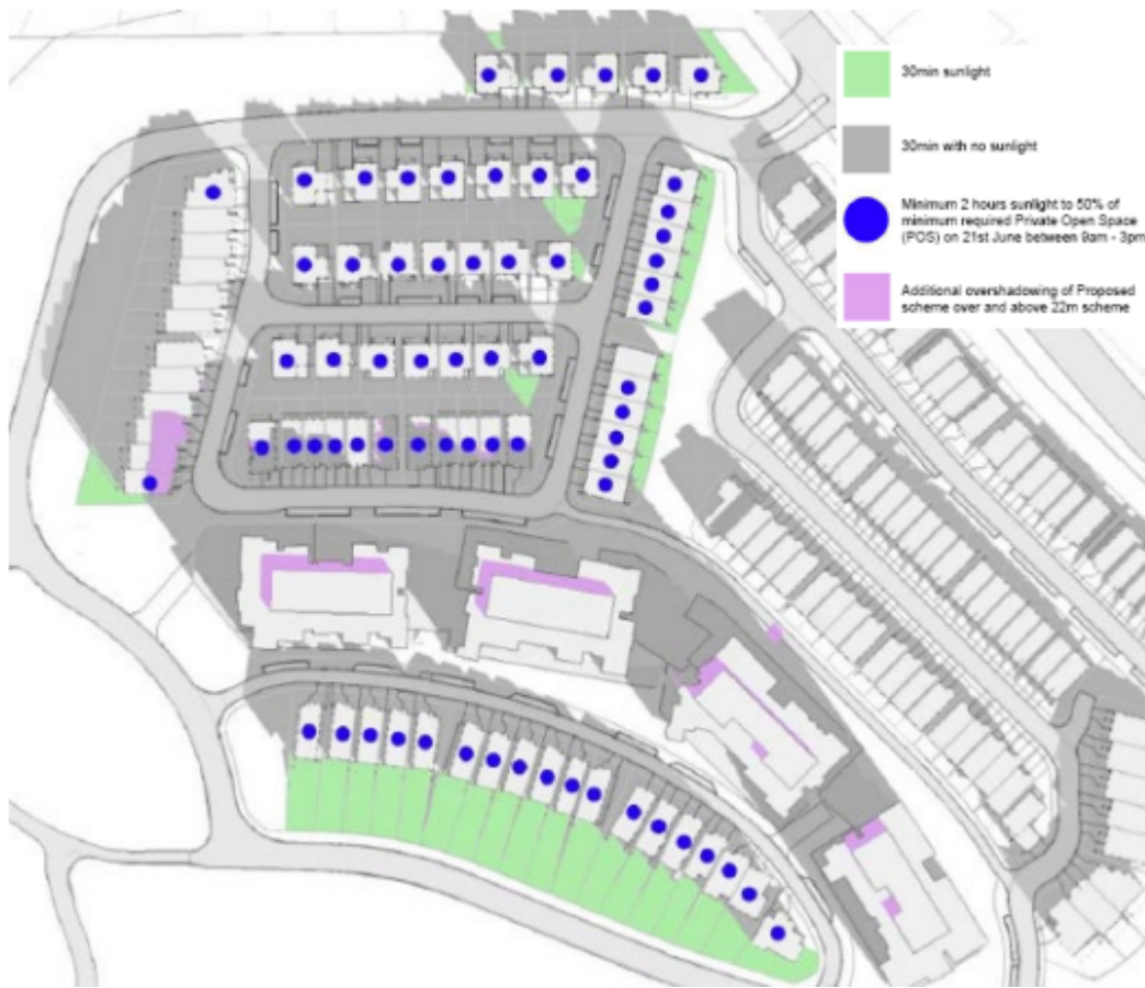
Figure 14: Shadow Diagrams at 9am on 21 June showing a compliant vs non-compliant (shown purple) development. Source: Mirvac Design
