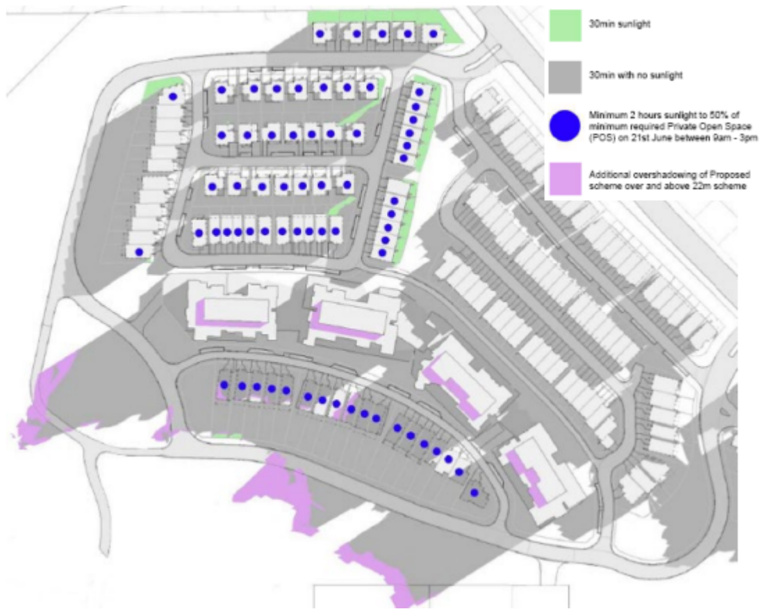
Figure 16: Shadow Diagrams at 3pm on 21 June showing a compliant vs non-compliant (shown purple) development. Source: Mirvac Design
