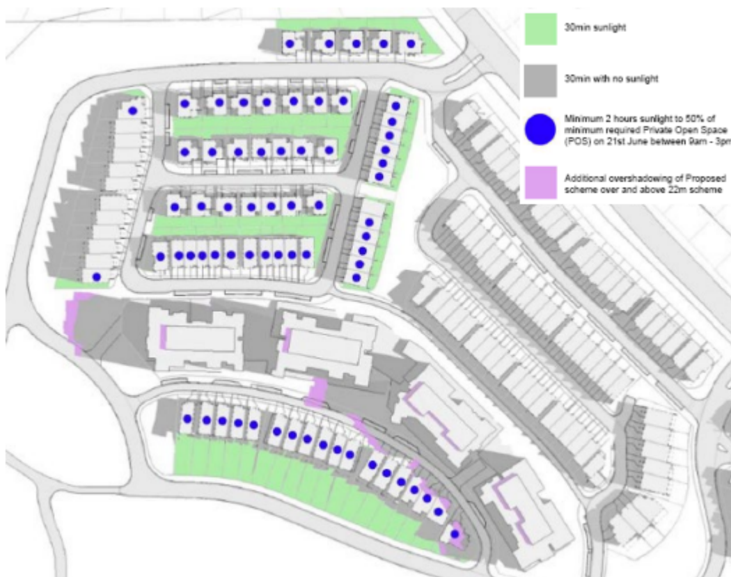
Figure 15: Shadow Diagrams at 12pm on 21 June showing a compliant vs non-compliant (shown purple) development. Source: Mirvac Design
